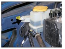
8. Remove the front P/S reservoir mounting bolt shown.
