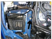
10. Install the provided short m/m rubber mounted studs into the airbox mounting location on the frame rail.
