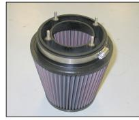
13. Install the filter adapter assembly into the K&N<sup>®</sup> air filter and secure with the provided hose clamp.
