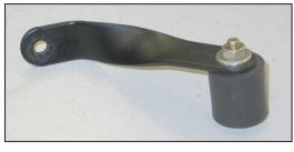
17. Install the long, m/f rubber mounted stud onto the heat shield mounting bracket (07139) as shown.
