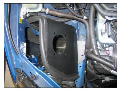
19. Install the heat shield assembly into the vehicle and secure to the rubber mounted studs with the hardware provided.
