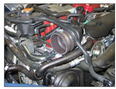
3. Remove the two clips that retain the fresh air inlet duct. Then remove the fresh air inlet duct from the vehicle.
