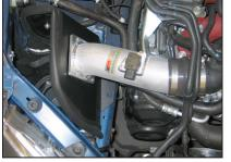
22. Install the K&N<sup>®</sup> intake tube into the silicone hose at the throttle body as shown.
