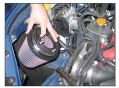
15. Set the filter assembly into the fender in preparation for the heat shield installation.
