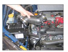
5. Remove the stock intake tube from the vehicle.
