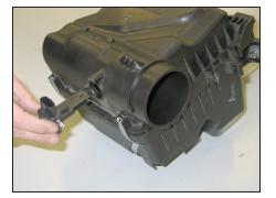
20. Remove the mass air sensor from the stock airbox as shown.
