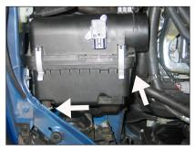
6. Remove the bolt and nut that secure the stock air filter housing.
