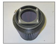
14. Install one of the provided gaskets onto the filter adapter as shown.
