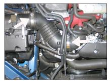
4. Loosen the two hose clamps that secure the stock intake tube.
