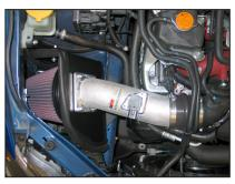
23. Install the filter so that the mounting studs pass through the heat shield, two gaskets, and intake tube flange and then secure with the provided hardware.
