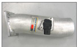
21. Install the mass air sensor into the K&N<sup>®</sup> intake tube and secure with the provided hardware.
