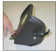
18. Install the heat shield mounting bracket assembly onto the heat shield as shown and secure with the provided hardware.
